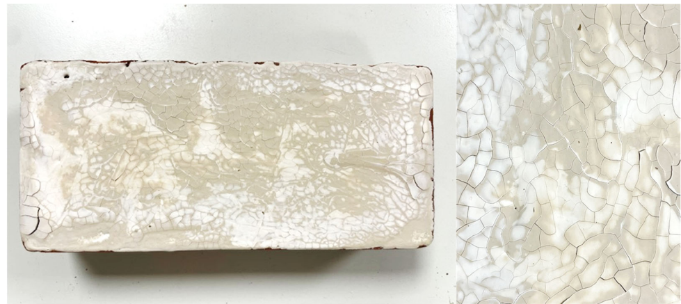
Figure 9. FA-0 thin layer applied on clay brick substrate.
