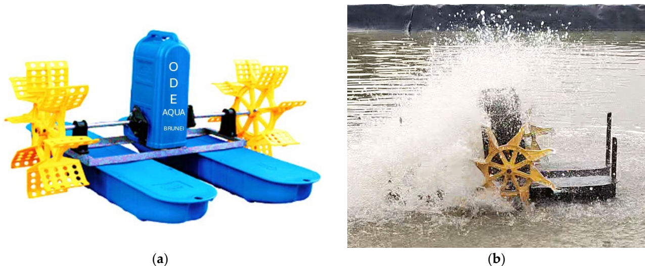
Figure 2. (a) Two-impeller wheel aerator; (b) operation of paddle wheel aerator.
