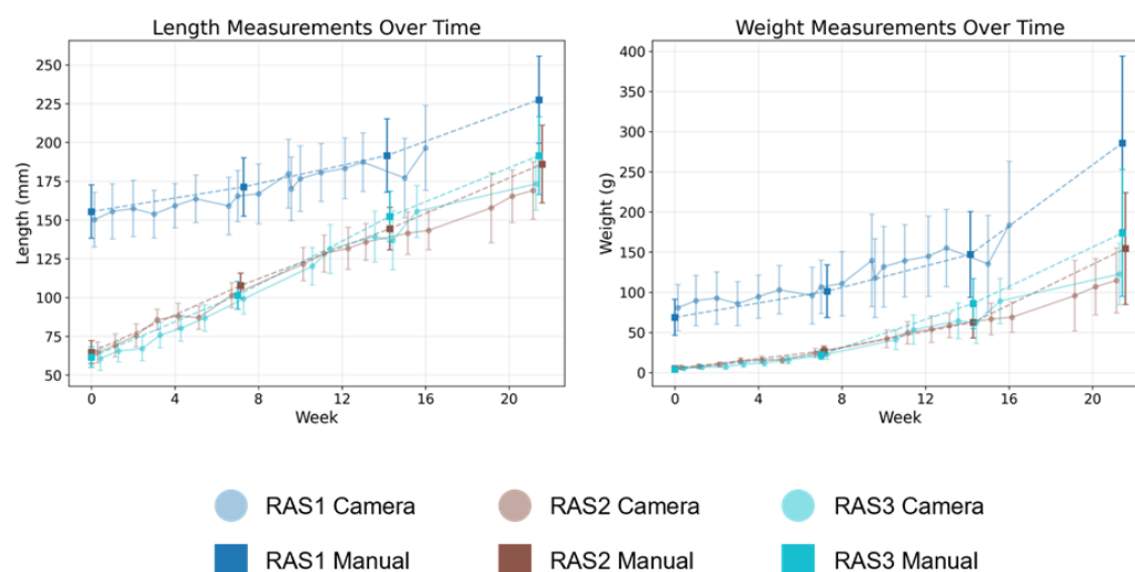
Figure 8. Growth curves of three fish populations cultivated in individual recirculating aquaculture systems (RAS1–3) over a 20-week monitoring period. Automated computer-vision-based measurements (solid lines) are compared with periodic manual reference measurements (symbols).
