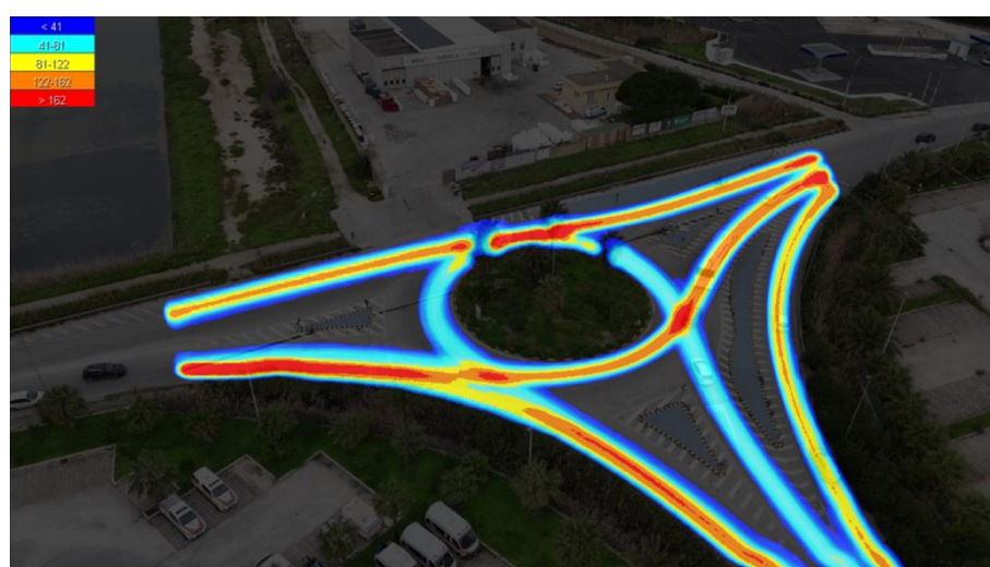
Figure 7. Heat map from UAV video-processing software.
