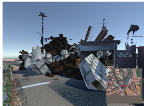
Figure 10. Physics-based building collapse and debris generation in Unity (RayFire).
