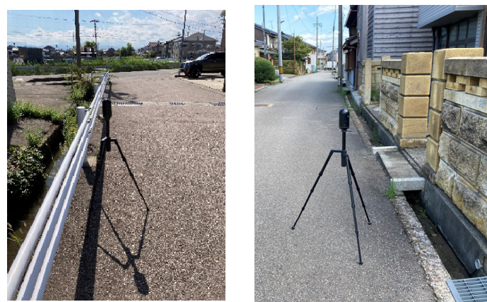
Figure 2. Field scene of the point-cloud survey (Leica BLK360 scanning procedure).
