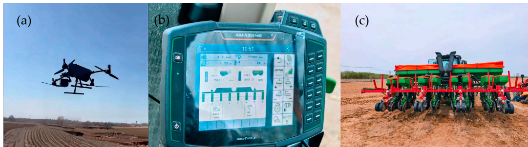
Figure 1. Map-based variable rate fertilization (VRF) system (a) UAV-based farmland quality assessment; (b) Execution of VRF prescription map (c) Working process of variable rate fertilizer applicator.
