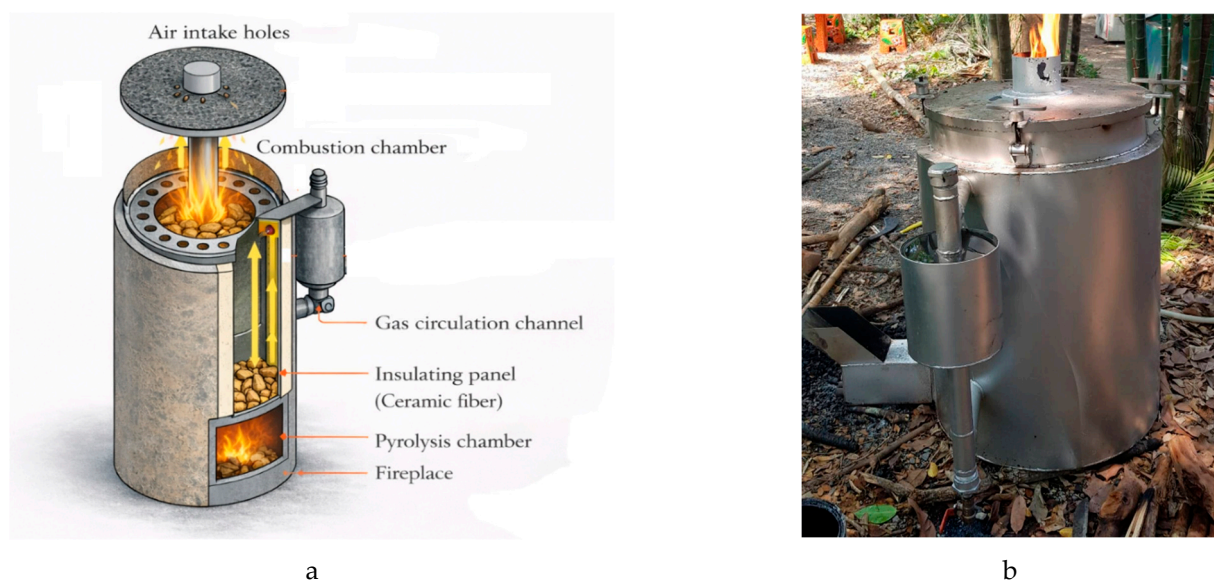
Figure 2. Schematic illustration and actual prototype of the smokeless vertical charcoal kiln: (a) schematic diagram showing the double-layer structure and gas circulation pathway for secondary combustion and heat recovery; (b) actual prototype of the kiln used in this study.
