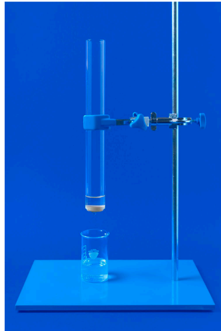
Figure 2. Xylem tissue water filtration. Photograph by Bor Cvetko, 2022; reproduced with permission.
