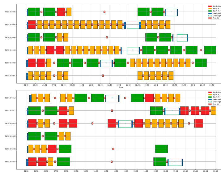
Figure 16. Schedules of partial electric buses for both types (TLH-EBS).
