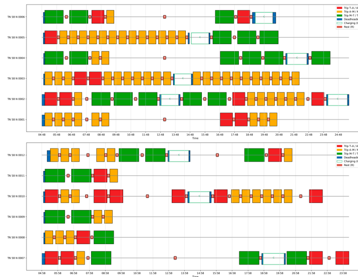
Figure 15. Schedules of partial electric buses for both types (RBS-LNS).
