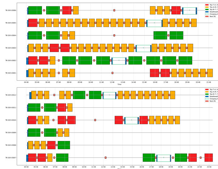
Figure 13. Schedules of partial electric buses for both types (MILP).
