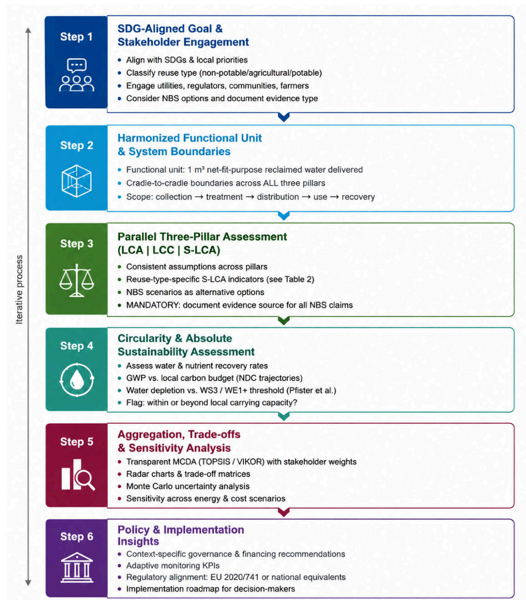
Figure 1. The RENEW-LCSA Framework: a six-step operational approach for urban municipal wastewater reuse. Steps are color-coded by functional cluster: blue (Steps 1–2) = scoping and boundaries; green (Steps 3–4) = assessment and absolute sustainability; red (Steps 5–6) = synthesis and policy translation. The iterative feedback arrow (left) indicates that later steps may require revisiting earlier ones. The framework is modular: Steps 1–3 may be applied first for preliminary scoping, with Steps 4–6 elaborated as data become available.
