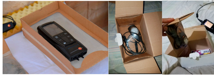
Figure 6. In situ surface reflectance measurement setup using a Testo 545 lux meter and a reference grey card.
