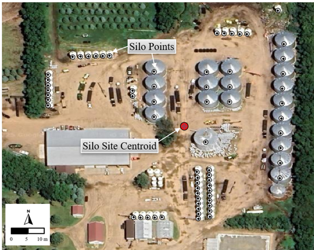
Figure 4. Cluster centroid representing a site containing numerous silo points.
