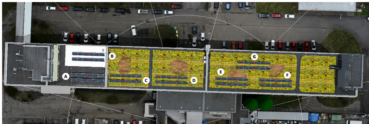
Figure 1. Rooftop layout and spatial zones used for assigning the nominal albedo scenarios in the PV*SOL model. Letters A–G denote the seven spatial roof zones used in the scenario analysis.
