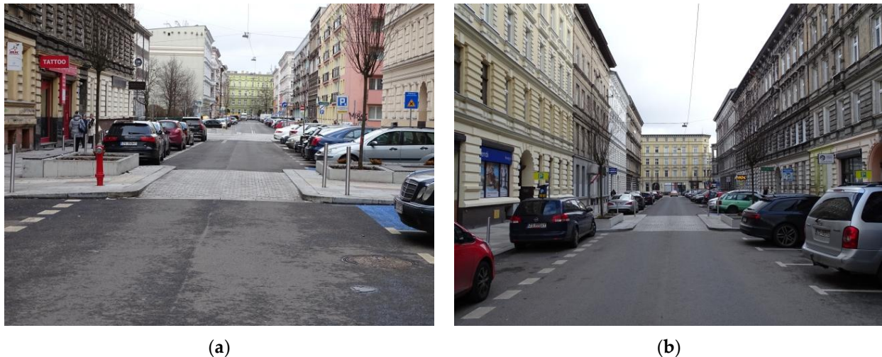
Figure 3. Raised mid-block narrowings: (a) one-way street section in Study Area 1, bollards followed by a concrete planter; (b) one-way street section in Study Area 3, a concrete planter followed by bollards. Source: photos by the authors.
