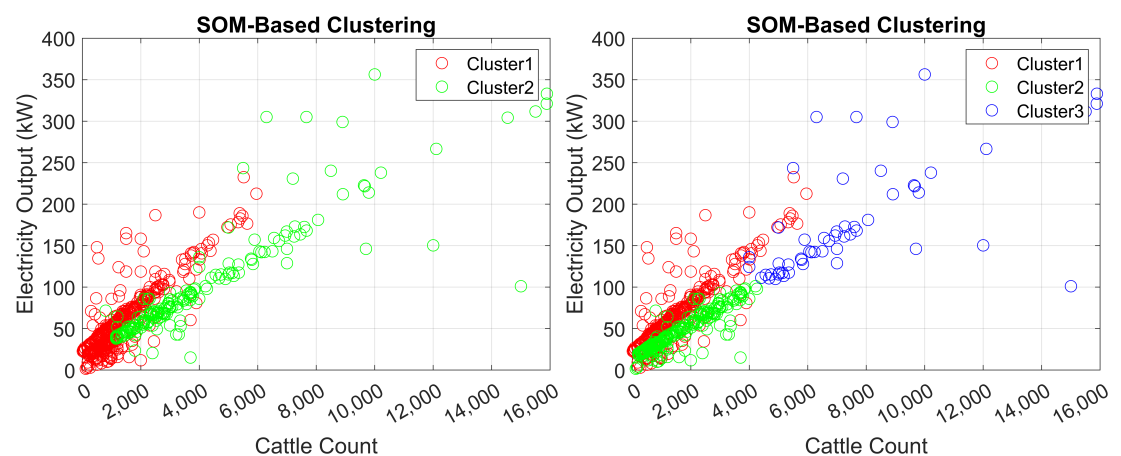
Figure 4. Comparison of SOM Clustering with 2 Clusters (left) and 3 Clusters (right). Overlap in the 3-cluster version introduces ambiguity and sparsity.
