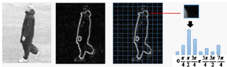
**Figure 3.** Using line edges to approximate the contour of an object.
