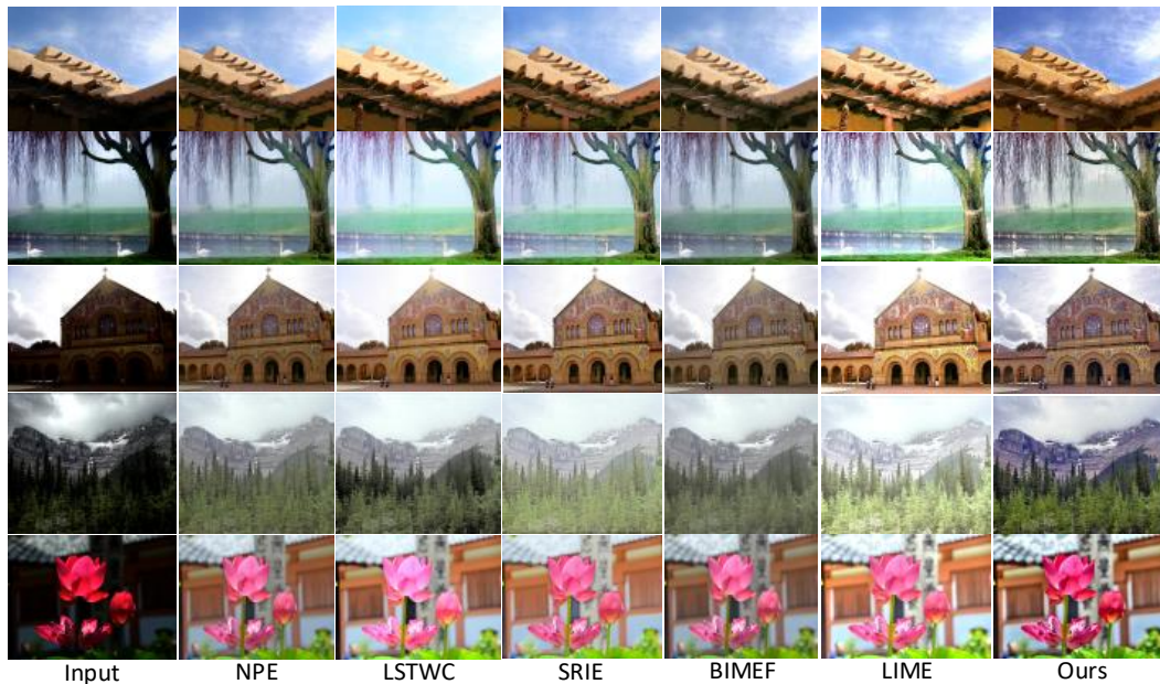
Figure 4. A comparison of the results of the handling of several visual artifacts. For example, in the first row, the sky color, clouds, wall texture, and dark regions were addressed. The haze and color were treated well in the images given in second row. The texture details, trees, and leaf colors were enhanced well in the images given in the third, fourth, and fifth rows, respectively.
