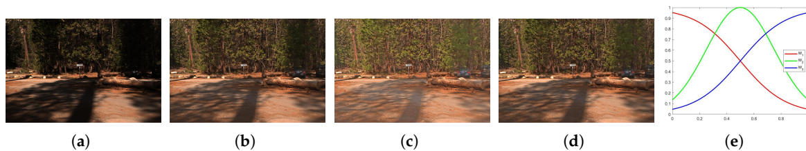
Figure 3. Multi-scale fusion process weights setting. (a) the original image; (b) the first enhanced image; (c) the second enhanced image; (d) the result of fusion; (e) the weight function.
