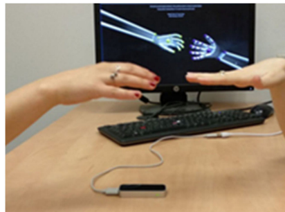
Figure 1. The participant and the research assistant sat on different sides of the table and were asked to move their hands above the Leap Motion depth sensor.
