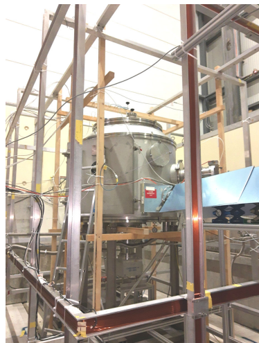
Figure 7. Photo of the experiment setup in the UCN area West during the test measurements in fall 2020. The visible parts can be compared with the description given in Figure 6. The UCN glass guides (on the right hand side) leading from beamport West-1 to the apparatus are covered by folded sheet metal pieces for protection. The visible metal frame supports the coil-windings, the wooden frame supports the fluxgates.
