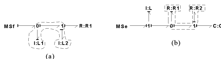
Figure A1. Bond graphs with (a) class 1 and (b) class 2 zero-order causal paths.
