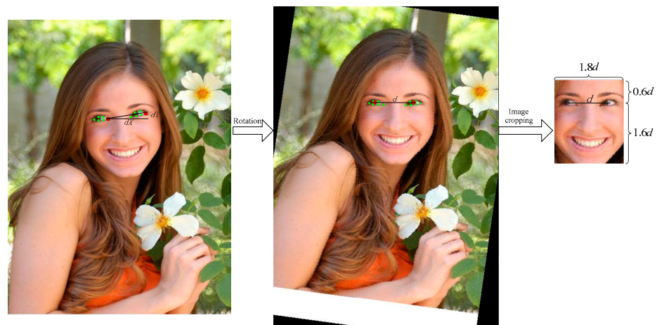
Figure 3. Face alignment and ROI_{face} cropping.
