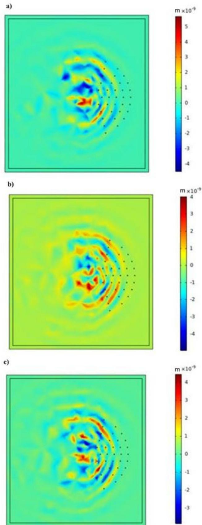
**Figure 6.** (a) In-plane displacement at a frequency of 6.5 Hz, (b) in-plane displacement at a frequency of 8.5 Hz, and (c) in-plane strain at a frequency of 14 Hz.
