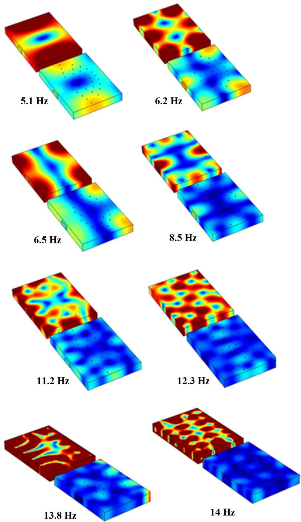
Figure 5. Total displacement areas in empty fields and air-filled boreholes at resonance frequencies.
