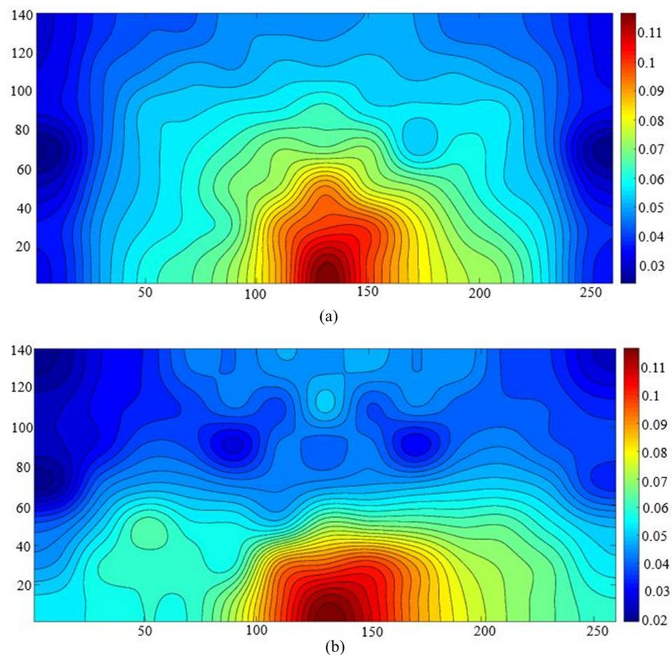
**Figure 9.** (a) Soil field at 6.5 Hz frequency. (b) Field where concrete piles at 6.5 Hz frequency are applied.
