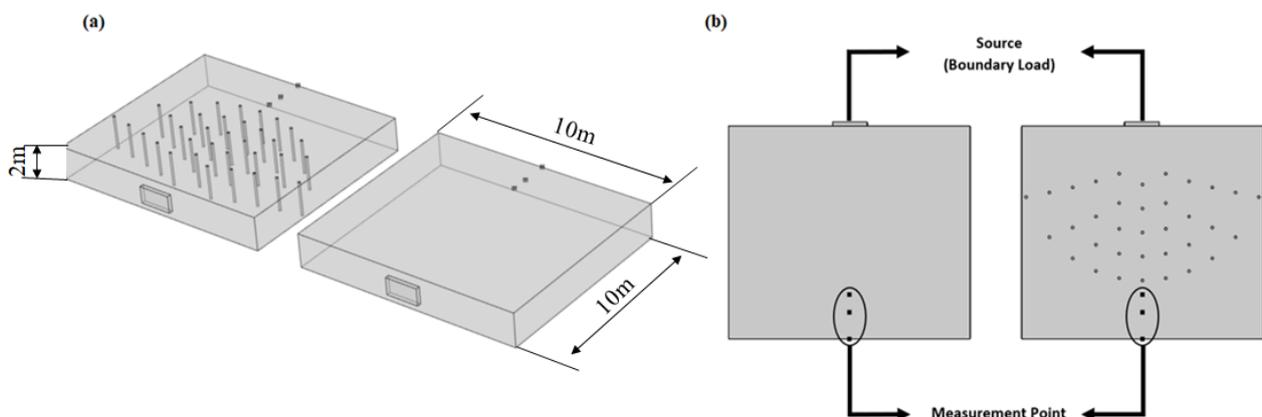
**Figure 2.** (a) Fields with and without metamaterial; (b) boundary loads and measurement points.
