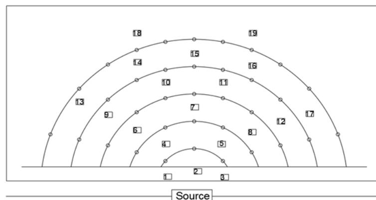
**Figure 8.** Locations of the accelerometers. The utilized number of the sensors are eighteen.
