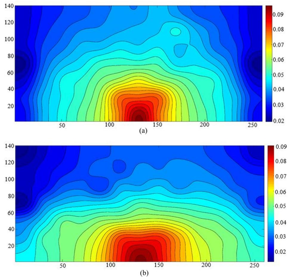
**Figure 10.** (a) Soil field at 8.5 Hz frequency. (b) Field where concrete piles at 8.5Hz frequency are applied.
