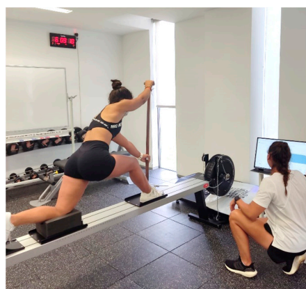
Figure 2. Specific adaptation of the Dansprint Canoe to the Functional Electromechanical Dynamometry cable for the incremental dynamometric test.
