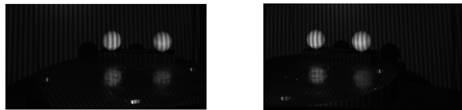
Figure 9. Phase map captured by left and right cameras.
