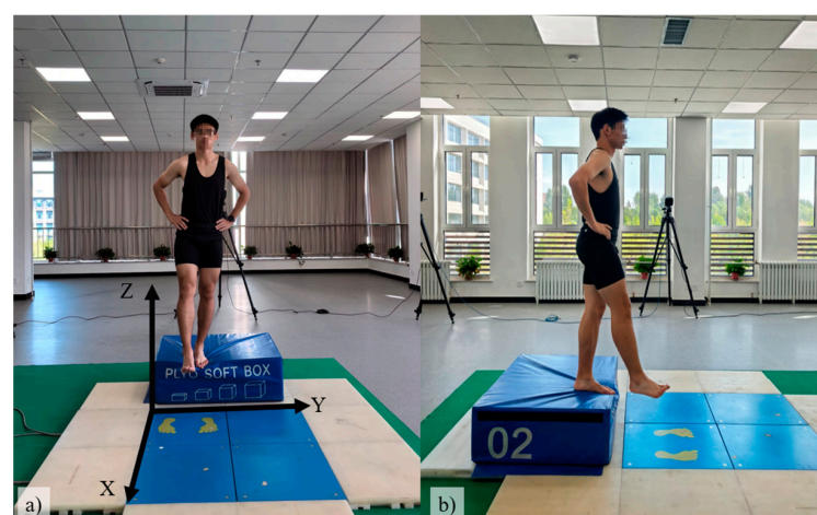
Figure 1. Setup of the single-leg landing postural stability test. (a) Front view; (b) Side view. X, Y, and Z indicate the force platform's anterior-posterior (AP), medial-lateral (ML), and vertical (V) directions, respectively.
