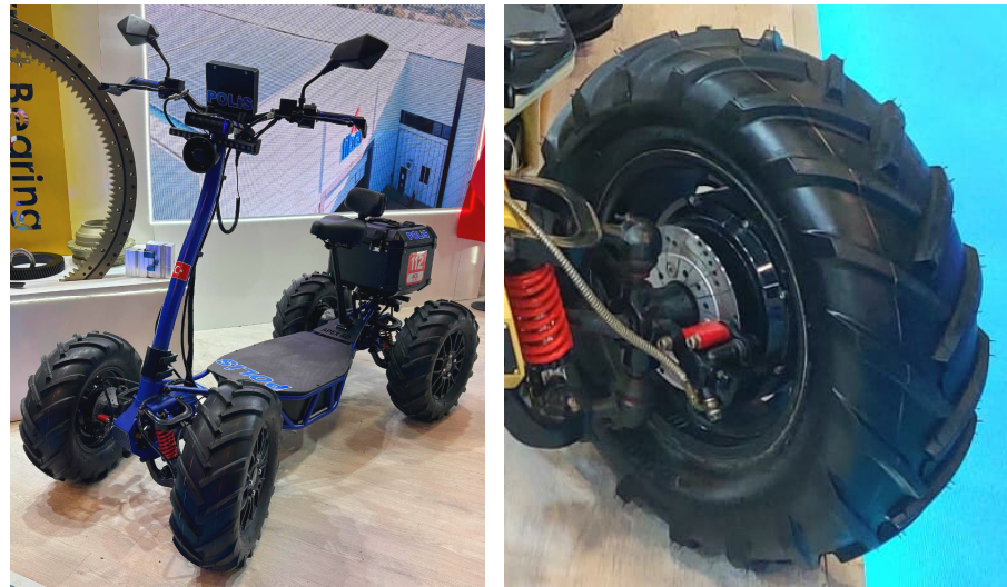
Figure 21. Prototype 4 × 4 electric scooter with independent suspension designed and manufactured within the scope of the study (Courtesy of Tibet Makine Sanayi ve Ticaret A.Ş.).
