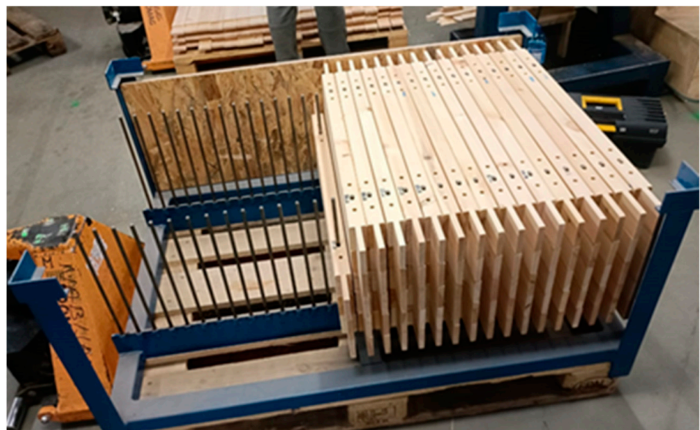
Figure 2. A jig for verifying claw nuts’ correct insertion and arrangement of holes in an asymmetrical furniture element.
