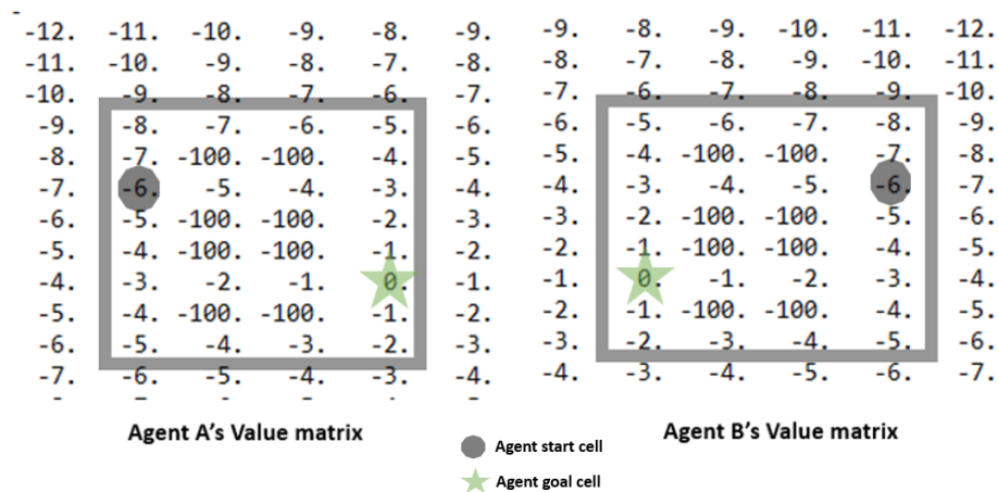
Figure 5. The Value matrix generated by the value iteration algorithm for Figure 4.
