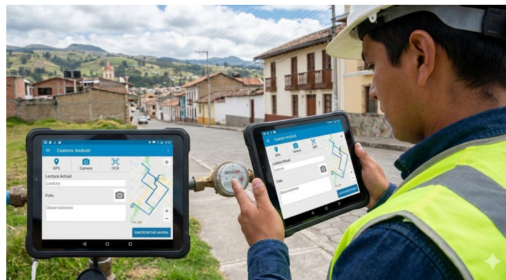
Figure 5. Example of a mobile meter-reading application for water utilities, used to capture field data directly from meters with geolocation and photo verification features.
