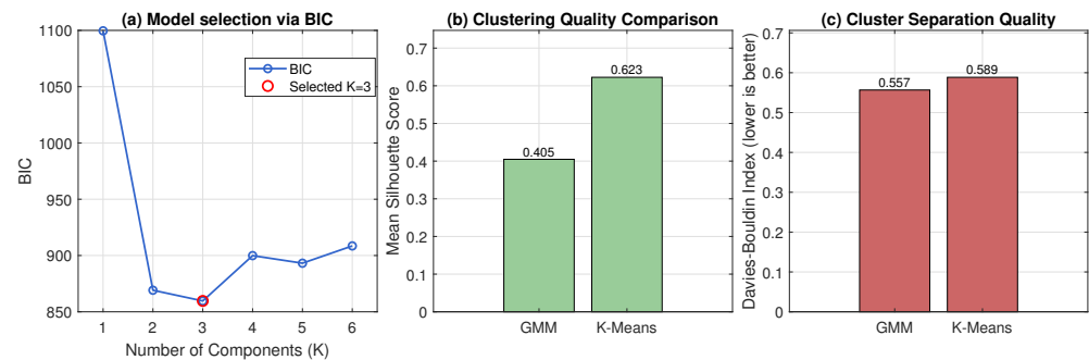
Figure 3. Model selection and clustering quality evaluation. (a) Bayesian Information Criterion (BIC) values for Gaussian mixture models with varying numbers of components, (b) comparison of mean silhouette scores between GMM and k-means clustering, and (c) Davies–Bouldin index comparison.
