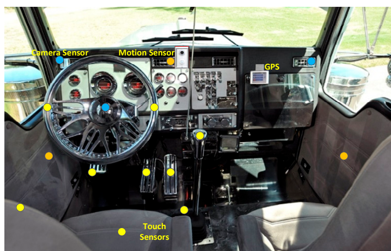
Figure 3. Sensor positions of vehicular information systems (Image adapted from Reference [13]).
