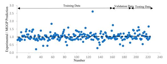
Figure 8. Experimental to MGGP-predicted bond strength rations.
