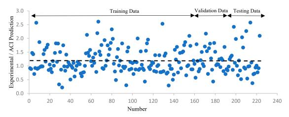
Figure 9. Experimental to ACI-predicted bond strength rations.
