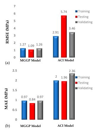
Figure 6. (a) RMSE of the MGGP and ACI models. (b) MAE of the MGGP and ACI models.
