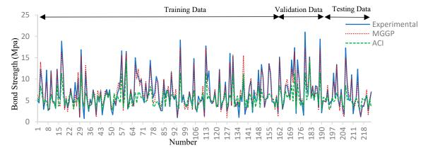
Figure 7. Bond strength predictions using the MGGP and ACI models.
