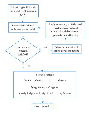
Figure 2. The MGGP block diagram.
