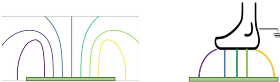
**Figure 2.** Approximate electric field lines in the case of loading mode capacitive sensing. If no object is present, the opposite parallel plate can be imagined to be in the infinity. When a human object is above the plate capacitor, the electric field lines will end on the foot as the opposite plate capacitor. Electric field lines are always orthogonal to the surface.
