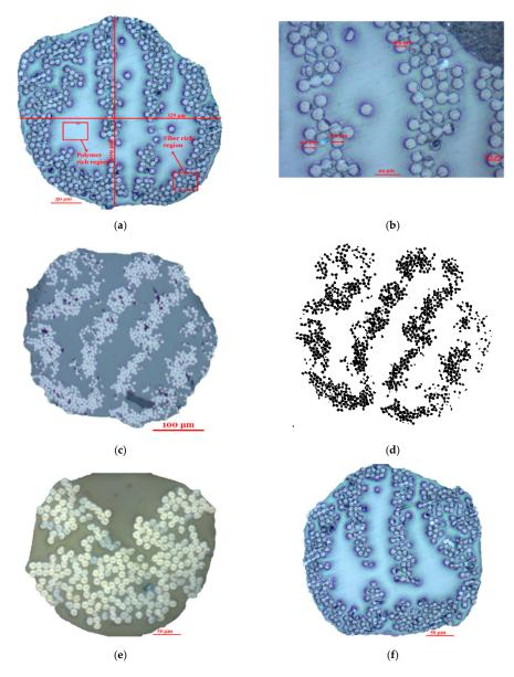
**Figure 4.** Cross-sectional views of fiber filaments (for fiber supply); fiberglass at  $200 \times (a)$ , fiberglass  $500 \times (b)$ , carbon fiber at  $100 \times (c)$ , carbon fiber filament tows shown as dots applying cell counting procedure using ImageJ (d), Kevlar at  $200 \times (e)$  and high strength high temperature fiberglass (HSHT) FG at  $200 \times (f)$ .
