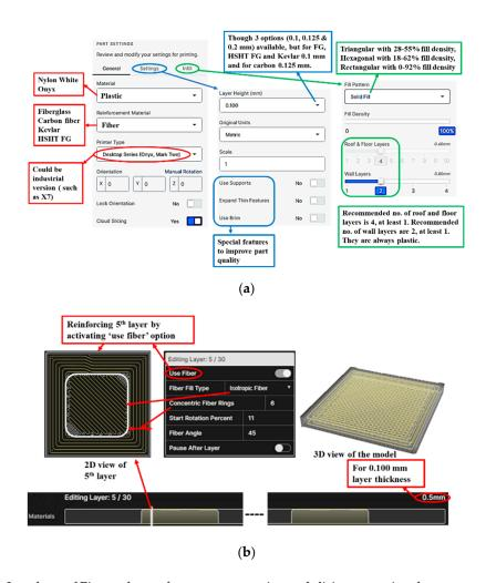
**Figure 5.** Interfaces of Eiger software for parameter setting and slicing: part view for parameter settings (**a**) and internal view for slicing as well as exploring different options for fiber-reinforcement (**b**).
