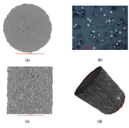
**Figure 3.** Different views of Onyx plastic filament: cross-sectional view from nano-CT scanning indicating fiber and void distribution (**a**), magnified (500×) microscopic view of the cross-section (**b**), longitudinal view from nano-CT scanning showing fiber orientation (**c**) and 3D view taken using nano-CT scanner (**d**).
