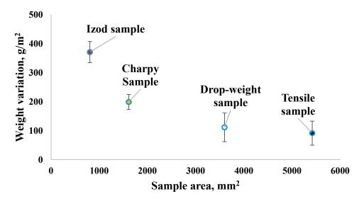
Figure 6. Variation in weights between estimated (by software) and measured for different sample sizes.
