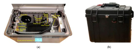
Figure 1. Mark Two 3D printer (desktop series) (a) and dry box to store and supply plastic filaments (b).
