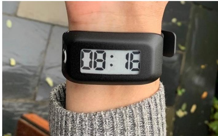
**Figure 6.** UMA Device with an integrated neural net for fall detection.
