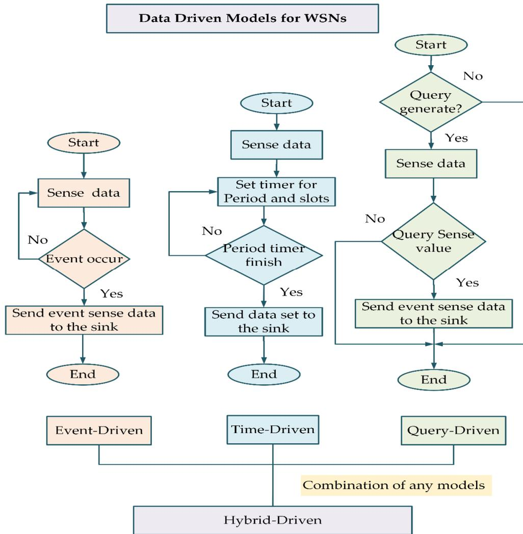
Figure 3. Process of data-driven models for WSNs.
