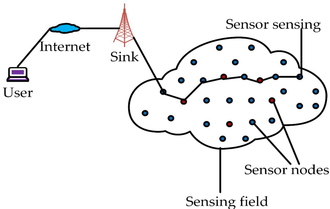
**Figure 1.** The typical network architecture of sensor nodes in a WSN.
