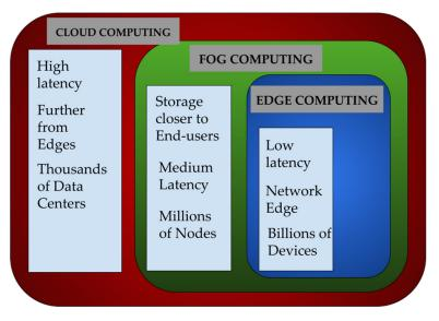
Figure 6. Hierarchical architecture and structural relationship between Cloud, Fog, and Edge computing.
