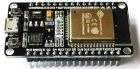
Figure 4. ESP-WROOM-32 development board.
