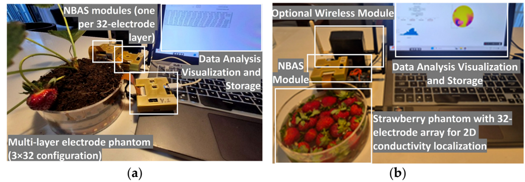
Figure 7. Tomography measurement setups: (a) 3D roots zone conductivity mapping; (b) 2D conductivity localization for postharvest fruit sorting.
