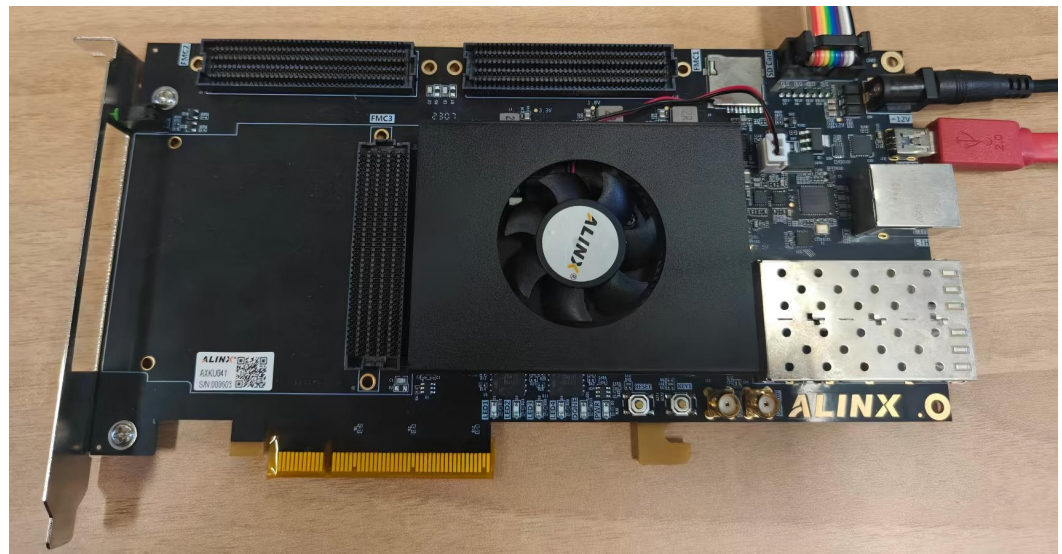
Figure 6. Photo of AXKU041 development board (Xilinx Kintex UltraScale) used for phasemeter hardware implementation and Doppler simulation experiments.
