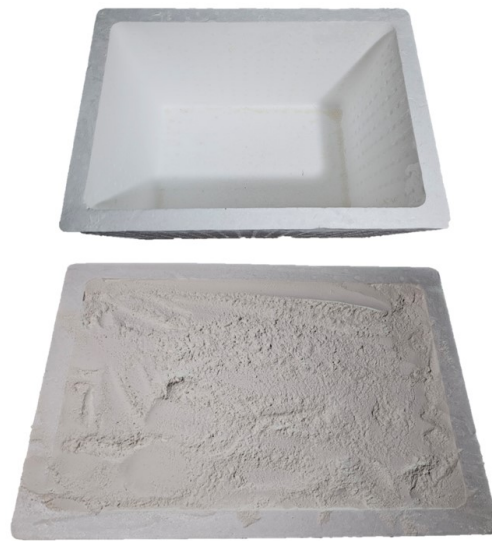
Figure 19. Container with a known volume used for testing. The container was utilized as a reference object to validate the accuracy of the system's volume estimation.
