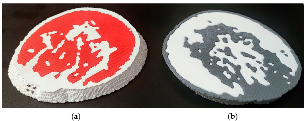
Figure 3. Pictures of the 3D-printed breast phantoms: (a) BP3 (ASA-HIPS, EP2) from the top side and (b) BP2 (ASA-ABS, EP1) from the bottom side. In (a) the adipose tissue (HIPS) is shown in red, whereas the glandular tissue and skin (ASA) are shown in white. In (b) the adipose tissue (ABS) is shown in white, whereas the glandular tissue and skin (ASA) are shown in gray.
