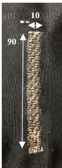
**Figure 1.** Layout of the embroidered sensor (dimensions in mm).
