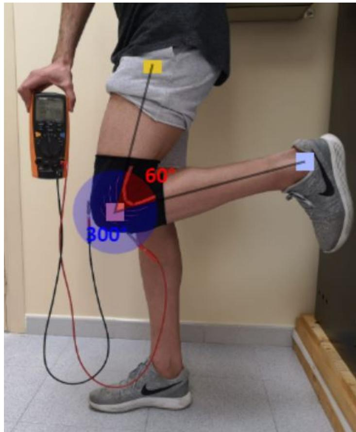
**Figure 5.** Characterisation of Knee flexion versus sensor resistance on kneepad.
