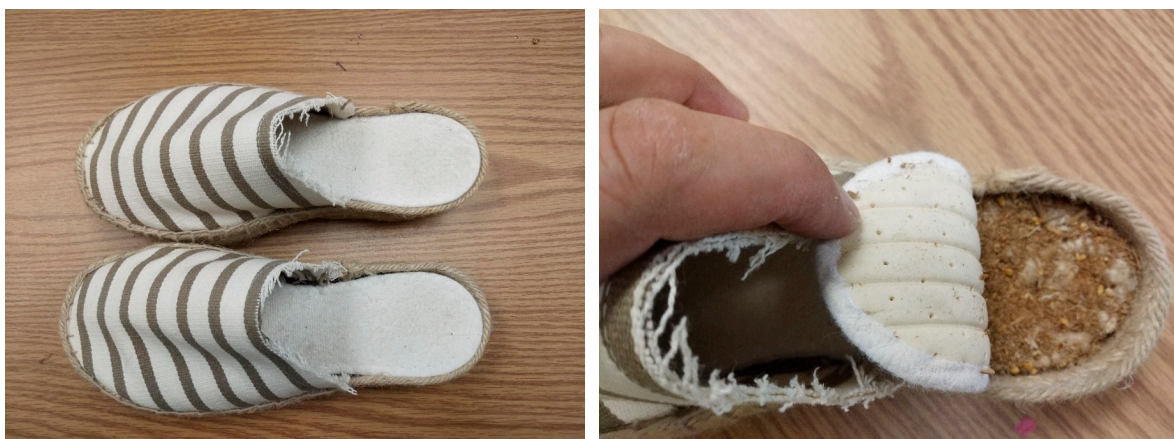
Figure 1. Shoe prototypes with mushroom mycelium composite as midsole ((left): shoe prototype; (right): the mycelium composite midsole).
