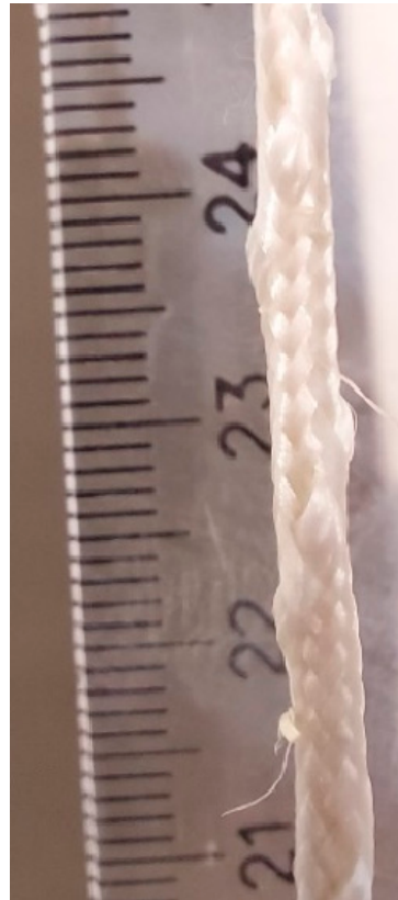
Figure 1. Sisal/PET braided yarn structure, sisal yarn in the core and 15 external single polyester plus one thicker binder yarn to improve bonding textile–matrix.
