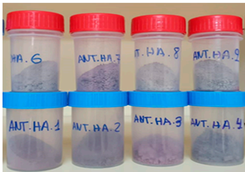
Figure 1. Images of the adsorption tests of anthocyanins in halloysite nanoclay.
