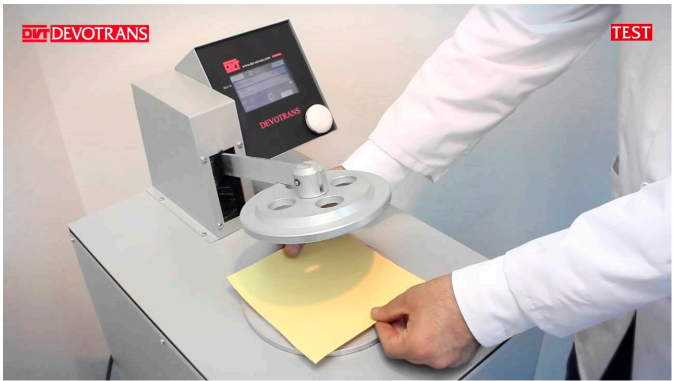
Figure 1. Devotrans HG DLC air permeability testing apparatus used in accordance with ASTM D737-04.
