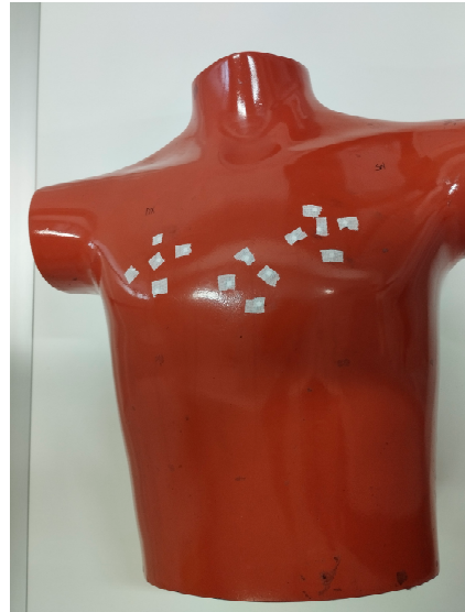
Figure 2. Positioning of the thermoluminescent dosimeters (TLDs) on the skin of the THOR phantom, indicating specific locations for lung (left and right) and heart dose measurements during both digital tomosynthesis (DTS) and traditional fixed-tube (RX) imaging modes.
