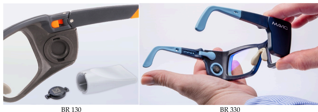
Figure 5. Radiation protection eyewear used for ocular dose monitoring with an integrated dosimeter attachment system.
